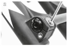
2. Tighten the safety clamp with a 4mm Allen wrench by suggested tightening torque of 7Nm.
