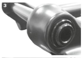
3. Check the axle's thread. It must be visible.
