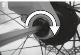
2. Tighten the axle with a 6mm Allen wrench by the suggested tightening torque of 8-10Nm.
