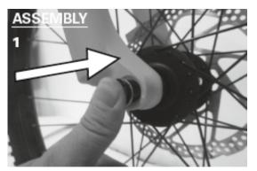
1. Fully insert the axle on the drive-side.
