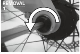
1. Loosen the axle on the drive side with a 6mm.
